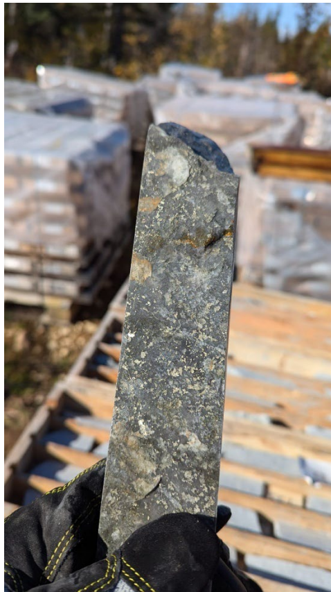
Photo 3: Drill core photo showing typical porphyry mineralization on the Property
